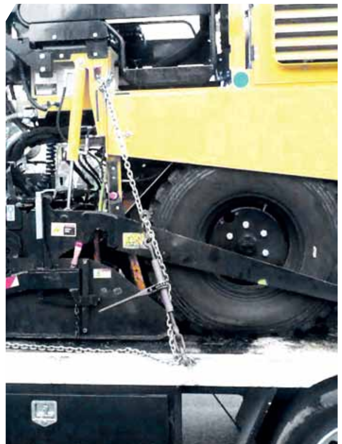
Turnbuckle type non-rebound tensioners have no kickback when released
