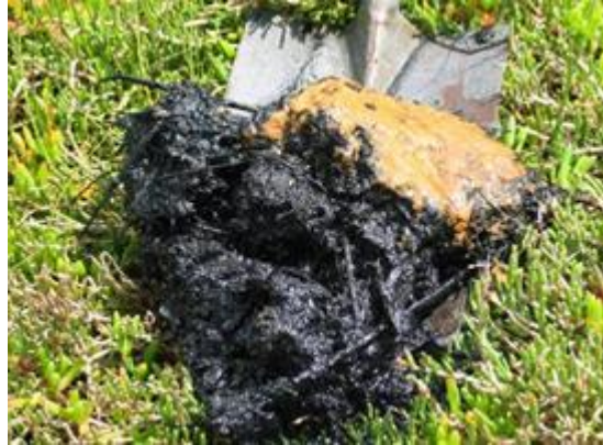
Exposed aggregate on a culvert in the Heart Morass. Dissolution of concrete structures helped detect disturbed CASS.
